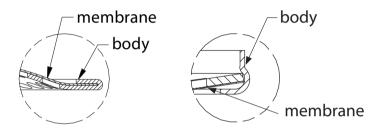
Its main feature is its very high filtering power of  $35 \mu m$  that guarantees a homogeneous distribution of water on the coffee pod and blocks the passage of extraction residue during the drying process. This helps to maintain the group as clean and efficient as when it was new. In addition, it protects both the group and the solenoid valve from deterioration caused by dirt.
