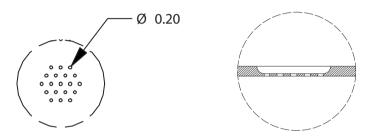
Its main characteristic is the exclusive design of its perforations, which, in addition to guaranteeing better distribution, makes this product last longer and easy to clean. Indeed, being made out of a single part, the shower body is more resistant and its surface is totally smooth and free from rough spots where dirt can deposit and accumulate.
