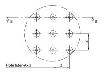
E: distance between holes of 1,73 mm distributed in a hexagonal pattern Maximum number of holes: 715 Within a maximum Ø of 49 mm
