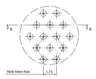
M: distance between holes of 1,50 mm distributed in a rectangular patter Maximum number of holes: 641 Within a maximum Ø of 44 mm
