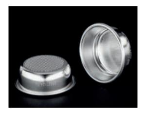
The filter shape with a rounded internal corner concentrates extraction towards the centre of the coffee puck, avoiding those sections where the ground coffee is not well utilised during the extraction process. This is combined with an M type of perforation that has a greater concentration of holes in a restricted area.
